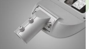
Powder painted aluminum cast housing highly weather proof. Luminaire is equipped with adjustable handle designed for mounting on posts and arms of 60 mm diameter. Level of tightness IP66. Diffuser is made of hardened glass. Following color temperatures are available: 4000 K. It is possible to program an autonomous multi-level or manual power reduction for specific customer needs by using a specialized power supply in the luminaire.
