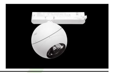
Elegant sphere-shaped projector. The housing is made of die-cast aluminum and the optics are a high-performance aluminum reflector. Different luminous flux variants and light distribution types are available. Adjustment mechanisms allow rotation of 355 degrees and tilting up to 90 degrees. Designed for lighting shop windows, art galleries and exclusive interiors.
