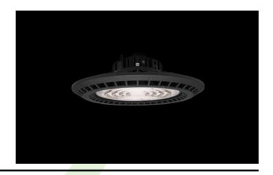
Industrial luminaire equipped with high performance LED sources. Mounting on pendants. Body made of cast aluminum, which also acts as a heat sink for LED modules. Powder coated in black (RAL 9005). The luminaire has a high degree of protection against dust and water ingress - IP65. Luminaires available with different light distribution: 60°, 90° and 120°. Application: halls, warehouses etc.
