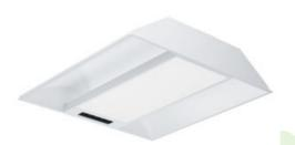
Luminaire designed to module suspended ceilings, equipped with the highly efficient LED panels. Luminaire body made from steel sheet, powder coated in white. The luminaire provides three different light distributions: main light distribution using micro-prismatic and smooth opal diffuser (during patient examination), indirect light distribution (during patient rest) and reading distribution using a louver.
