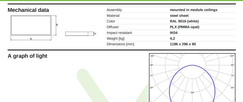
Luminous flux tolerance +/- 10%. Power tolerance +/- 10%. Technical data may be changed. Photos of the luminaires may differ from reality. Date of last update: 22-08-2025
