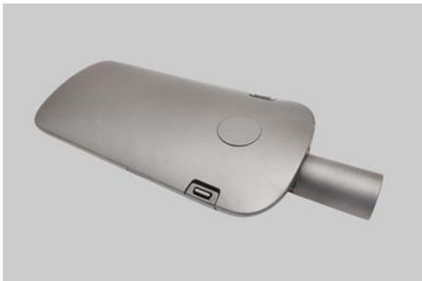
Powder painted aluminum cast housing highly weather proof. Luminaire is equipped with adjustable handle designed for mounting on posts and arms of 60 mm diameter. Level of tightness IP66. Diffuser is made of hardened glass. Following color temperatures are available: 5700 K.
