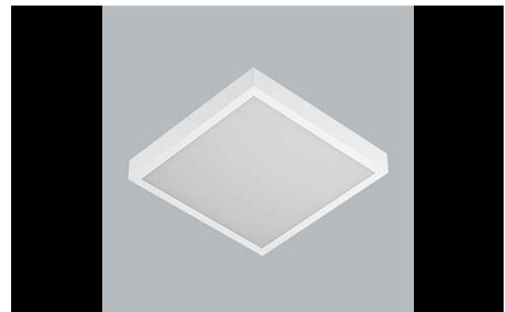
Surface mounted luminary equipped in highly efficient LED panels. Luminary body made from steel sheet, powder coated in white. Diffusers permanently mounted, no aluminum frame. Luminary recommended for: emergency departments, intensive care units, and treatment rooms.
