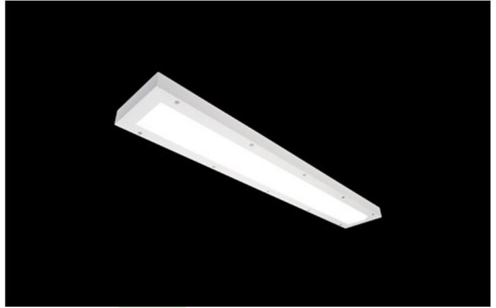
Surface mounted LED luminaire. Luminaire body made from steel sheet, powder coated in white. Luminaire 40 J impact resistant. Luminaire recommended for rooms of vandal and humidity hazards.
