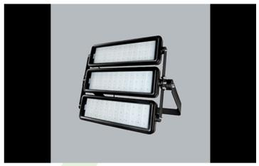
Numancia Arena delivers high-efficiency lighting for large-scale outdoor spaces, offering efficiency of up to 196 lm/W. Built for extreme temperatures (-40°C to +40°C) and durable with IP66 and IK09 ratings, it ensures reliable performance in challenging environments. Versatile beam options and high-quality optical systems make it a perfect choice for large sports arenas and other outdoor facilities.
