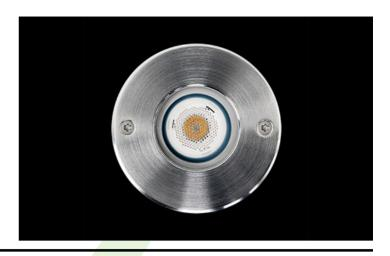
Designed for inground installation. Body built in die-cast aluminium with the frontal made of tempered glass and stainless steel finished in polish steel. Luminaire is IP67 and IK08. Luminaire built-in an optical system based on synthetic material lenses with an angle beam of 20°.
