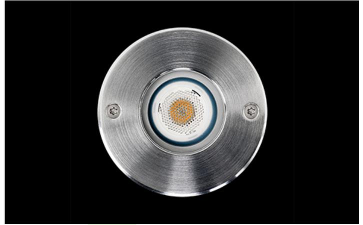
Designed for inground installation. Body built in die-cast aluminium with the frontal made of tempered glass and stainless steel finished in polish steel. Luminaire is IP67 and IK08. Luminaire built-in an optical system based on synthetic material lenses with an angle beam of 20°.
