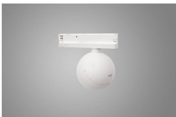
Elegant sphere-shaped projector. The housing is made of die-cast aluminum and the optics are a high-performance aluminum reflector. Different luminous flux variants and light distribution types are available. Adjustment mechanisms allow rotation of 355 degrees and tilting up to 90 degrees. Designed for lighting shop windows, art galleries and exclusive interiors.
