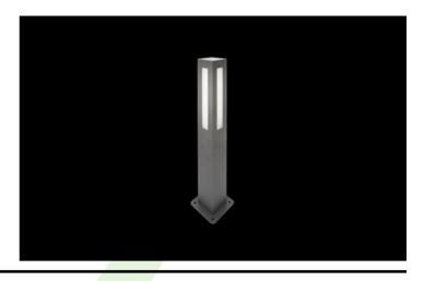
Outer luminary to be mounted on a solid surface (concrete, sett, or substructure) equipped with highly efficient energy saving LED sources of the newest generation. Luminary dedicated to illuminate pedestrians routes such as park alleys, parking site passages, property entrances. Its body made from aluminum (profile size 100x100mm) which is coated by the facade powder used for outdoor activities. PLX opal diffuser
