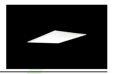
Modern LED panel for installation in suspended ceilings or directly on the ceiling. Equipped with the highly efficient LED sources. Luminary body made from aluminum. PMMA opal diffuser. Colour of luminary white. Luminary dedicated for the public use structure like offices, conference rooms, classrooms, lecture halls etc. The level of protection against solid substances, dust and moisture penetration is IP65.
