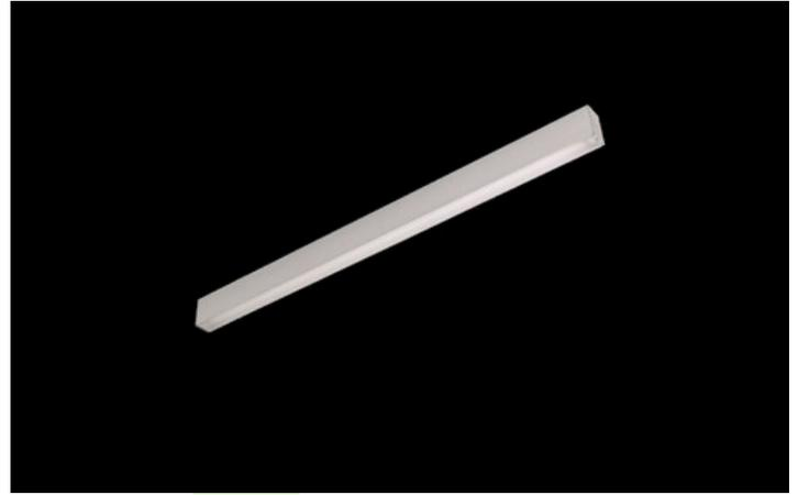
Luminaire made from aluminum profile adapted to be mounted on suspensions, or directly on a solid ceiling construction. Its body made from anodized aluminum profil. There are two colors available: white (RAL9016) or grey (RAL9006). Its diffuser is made from white polymethyl methacrylate. Luminaire to be used in offices, conference halls, all structures of public sectors.
