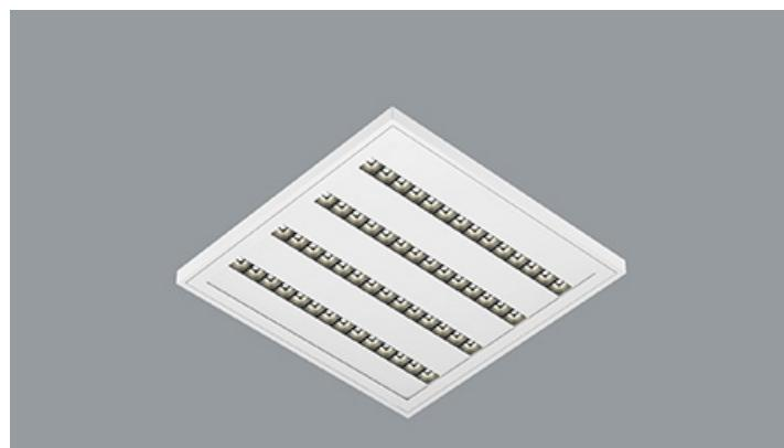
Surface mounted luminary. Equipped with highly efficient LED light sources. The Domino Clean Surface LOW UGR LED uses an anti-glare louvre which reduces glare and directs light precisely. Housing made of steel sheet. Significant diversity of the value of luminous flux. Colour rendering index CRI: 80. Level of tightness IP65.
