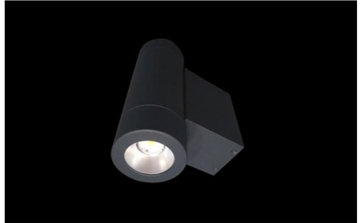
Luminaire adapted to be mounted on walls. High lighting efficiency LEDs were used. Its body is made from anodized aluminum profile. It is resistant to solids, dust, and liquids penetration – IP65. This type of luminaire is recommended for decorative or accent illumination of buildings.
