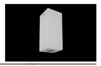
Decorative luminary of 1,5 W, and IP40 dust and water protection class. It is made from powder coated aluminum (RAL9006 standard). The standard light distribution is achieved owing to  $\pm 5^{\circ} x \pm 21^{\circ}$  lens. It is also possible to use the symmetric light distribution of 45°. Luminary designed for accent and decorative illumination in such areas as restaurants, pubs, or cafés.
