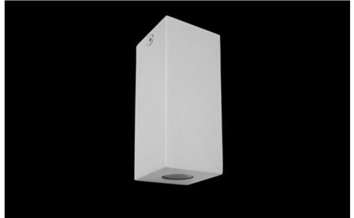
Decorative luminary of 1,5 W, and IP40 dust and water protection class. It is made from powder coated aluminum (RAL9006 standard). The standard light distribution is achieved owing to  $\pm 5^\circ \times \pm 21^\circ$  lens. It is also possible to use the symmetric light distribution of  $45^\circ$ . Luminary designed for accent and decorative illumination in such areas as restaurants, pubs, or cafés.
