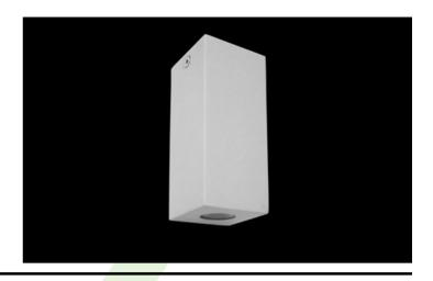
Decorative luminary of 1,5 W, and IP40 dust and water protection class. It is made from powder coated aluminum (RAL9006 standard). The standard light distribution is achieved owing to  $\pm 5^{\circ} x \pm 21^{\circ}$  lens. It is also possible to use the symmetric light distribution of 45°. Luminary designed for accent and decorative illumination in such areas as restaurants, pubs, or cafés.
