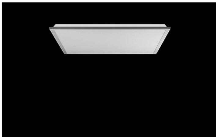
Modern LED panel dedicated to be mounted on suspended modular ceilings, cardboard suspended ceilings (using adaptive frame), directly on the ceiling (using adaptive frame) or using adaptive frame and suspensions. Equipped with the highly efficient LED sources. Direct light distribution. Luminary body made from steel sheet. PMMA opal diffuser. Colour of luminary - white. CRI>80. Luminary dedicated for the public use structure like offices, conference rooms, classrooms, lecture halls etc.
