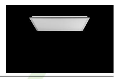
Modern LED panel dedicated to be mounted on suspended modular ceilings, cardboard suspended ceilings (using adaptive frame), directly on the ceiling (using adaptive frame) or using adaptive frame and suspensions. Equipped with the highly efficient LED sources. Direct light distribution. Luminary body made from steel sheet. PMMA opal diffuser. Colour of luminary - white. CRI>80. Luminary dedicated for the public use structure like offices, conference rooms, classrooms, lecture halls etc.
