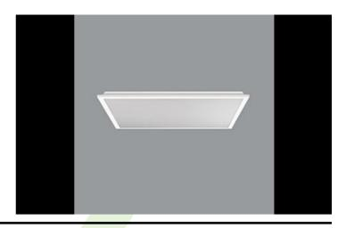
Modern LED panel dedicated to be mounted on suspended modular ceilings. Equipped with the highly efficient LED sources. Direct light distribution. Luminary body made from steel sheet. Micro-prismatic diffuser PMMA. Colour of luminary - RAL 9016 (white). CRI>80. Luminary dedicated for the public use structure like offices, conference rooms, classrooms, lecture halls etc.
