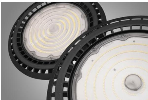
Industrial luminaire equipped with high performance LED sources. Mounting on pendants. Body made of cast aluminum, which also acts as a heat sink for LED modules. Powder coated in black (RAL 9005). The luminaire has a high degree of protection against dust and water ingress - IP65. Luminaires available with different light distribution: 60°, 90° and 120°. Application: halls, warehouses etc. The luminaires are not compatible with the Helvar control system.
