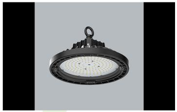
The Atena HT Industry luminaire delivers powerful, energy-efficient lighting tailored for the toughest industrial environments. Perfect for high-temperature facilities or cold storage, it operates flawlessly from -40°C to +70°C, offering up to 35,142 lumens with exceptional efficiency of nearly 160 lm/W. Built to last, it features IP65 and IK08 protection, providing reliable, high-performance lighting.
