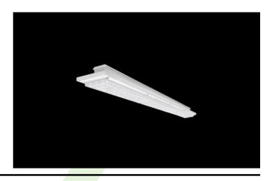
Agaline 3R is a single linear luminaire designed for mounting on slings. The body is made of white powder-coated steel sheet. Optical system based on lenses providing different light distribution. High level of protection against penetration of dust and water - IP65. Agaline is an excellent solution for lighting industrial facilities and warehouses, but also finds application in offices, supermarkets and shops.
