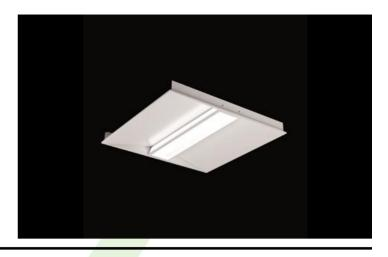
Luminary body made from steel sheet powder coated in white. Luminary adapted to be mounted in 600x600 module ceilings and with adaptive frame in plasterboard ceilings. It is equipped with highly efficient LED sources of the newest lighting generation, with the average durability of 60000 h. Diffuser is made from polymethyl methacrylate with micro prism structure (micro prism part of diffuser is the outer side of the luminary). Luminary resistant to solids, dust, and liquids penetration (IP20).
