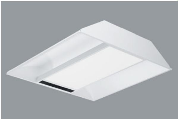
Luminaire designed to module suspended ceilings, equipped with the highly efficient LED panels. Luminaire body made from steel sheet, powder coated in white. The luminaire provides three different light distributions: main light distribution using micro-prismatic and smooth opal diffuser (during patient examination), indirect light distribution (during patient rest) and reading distribution using a louver.
