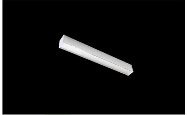
Light fitting made out of aluminium profile equipped with opal diffuser or MPRM and driver. X-LINE fittings are intended to be mounted on ceiling or pendants. In the family of X-LINE LED fittings modules of renowned brands are applied. The luminaire is equipped with LED modules adjusted to regulate the color temperature of light in the range from 2700 K to 6500 K.
