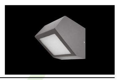
Powder painted steel housing. Possibility of mounting emergency module. Isolated battery applied in luminaire is equipped with thermostat enabling performance in low temperature up to -25° C. Updoor Mini might be mounted on walls or ceilings and is recommended to illuminate buildings' entrances, arteries, tunnels, underground entrances, etc.
