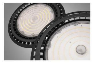
Industrial luminaire equipped with high performance LED sources. Mounting on pendants. Body made of cast aluminum, which also acts as a heat sink for LED modules. Powder coated in black (RAL 9005). The luminaire has a high degree of protection against dust and water ingress - IP65. Luminaires available with different light distribution: 60°, 90° and 120°. Application: halls, warehouses etc.
